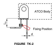
TABLE TK-3 Distance between Body and Bending Point
